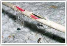
Gnawing on wires can result in fires.\*
